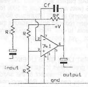
The supply voltage in this case could be anything between 5V and 15V. R<sub>i</sub> will be the input resistance and could be made equal to the output impedance of the microphone or any other desired value.
